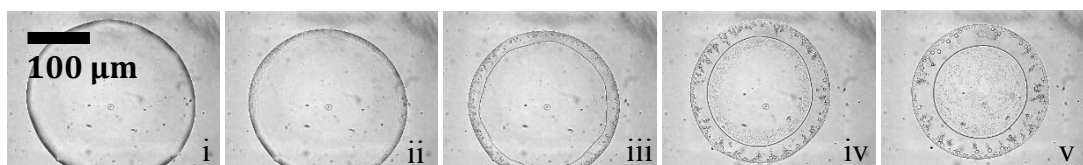
Figure C1. Images of evaporation of 3-methyl adipic acid - ammonium sulfate ternary aqueous solution droplet with OIR 2:1 on a glass-slide.
