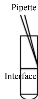
Fig 4.17 Way to add another solvent to create density gradient
