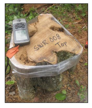
**Figure 3.6**: Cut and wrapped red pine stump sample with GPS for scale.
