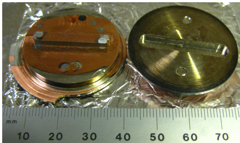
Figure 2.8: The chuck for adjusting inplane rotation (left) and the back of the growth platen (right).
