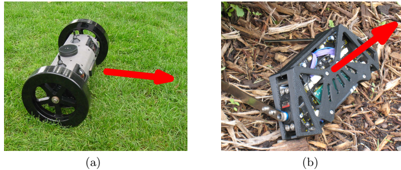
Figure 3.7: Figure depicting the ability of tumbling robots to aim rigidly attached directional sensors using the same actuators employed to generate locomotion. Sensor direction is represented by the red arrows. (a) shows a MegaScout with its sensor constrained to \mathbb{R}^2 while the Adelopod of (b) can point its sensor along vectors in \mathbb{R}^3 .
