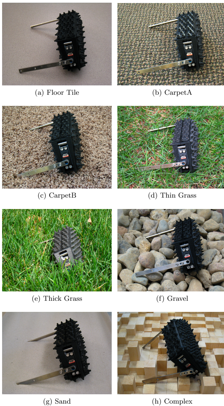
Figure 5.18: Experimental terrains with Adelopod posed for size reference.
