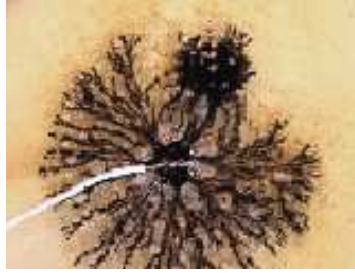
Figure 2.8 Schematic showing dendritic shape of a growing crystal [51]
