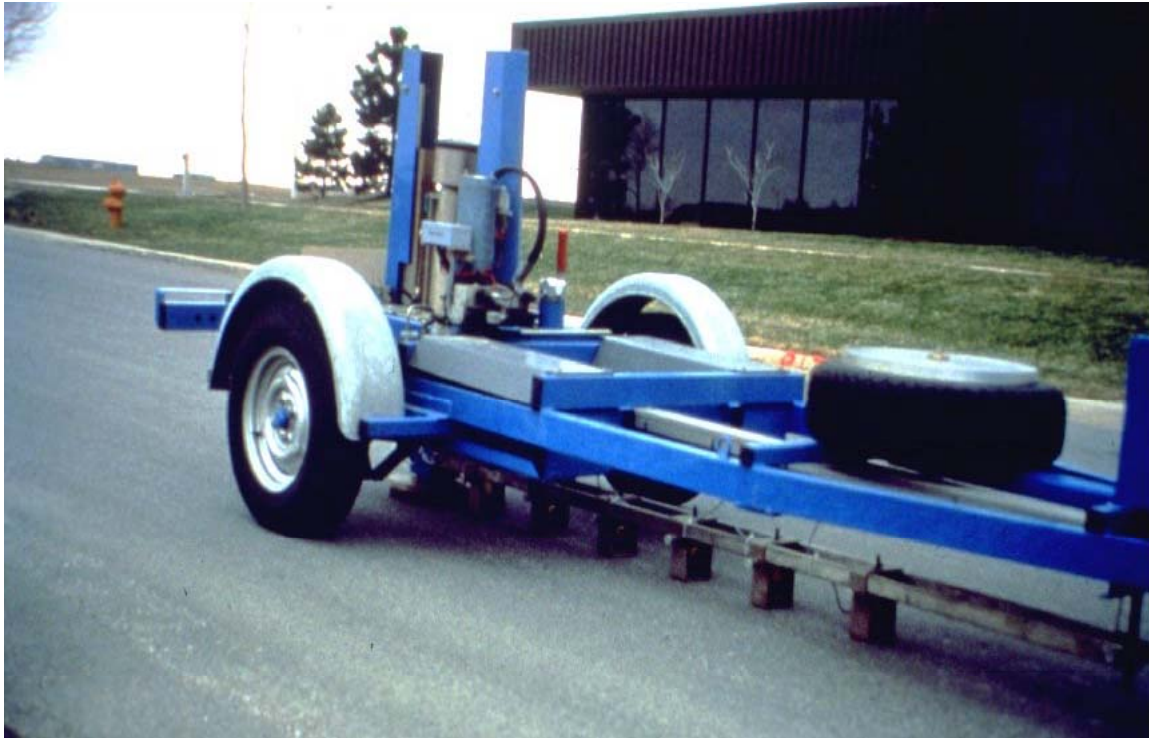
Figure 2-1 Photograph of a Dynatest Falling Weight Deflectometer
