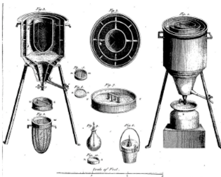
Figure 1.4: A view of the calorimeter. The left hand image shows a cross section of its interior. The right hand illustration depicts its outer casing. The middle images, from upper to lower, show the apparatus from above and at an angle. 148
