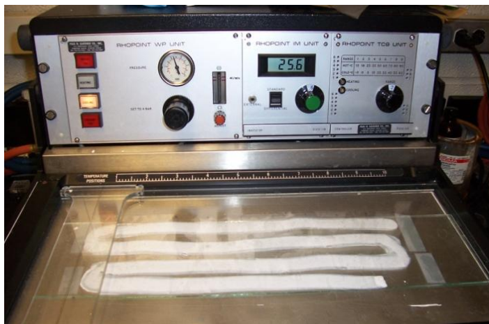
Figure 3.11 Minimum film formation temperature bar used in this report to efficiently produce samples at a range of temperatures. Samples are drawn down using a 0.75 \mu\text{m} cube applicator onto a metal bar. A temperature gradient is maintained down the length of the bar and 4 L/min of air is blown across the coating according to ASTM standard D2354.
