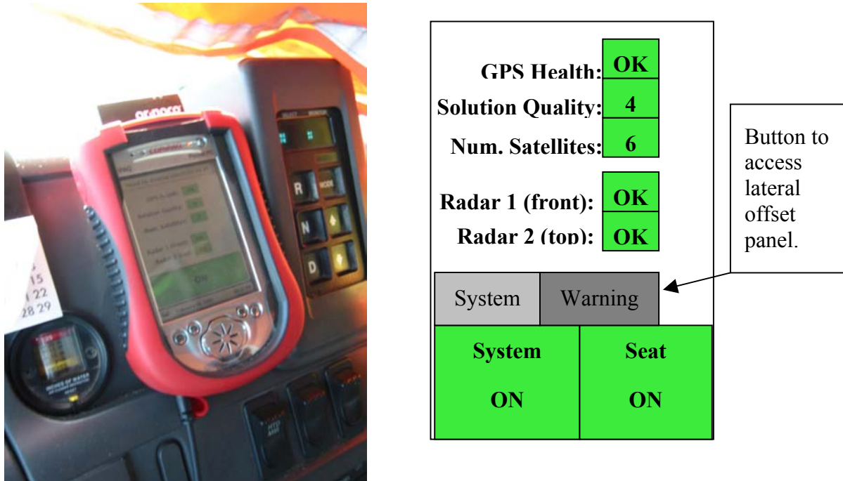
Figure 3.4. Primary display page of the iPAQ-based driver control panel for the driver assistive system. The vehicles evaluated in this project did not have active seats, so the button on the lower right of the display was a “dummy.” This page provides the driver information regarding the operational status of the system. The “Warning” button activates a panel which allows operator to select desired lateral offset. (See Figure 3.5).
