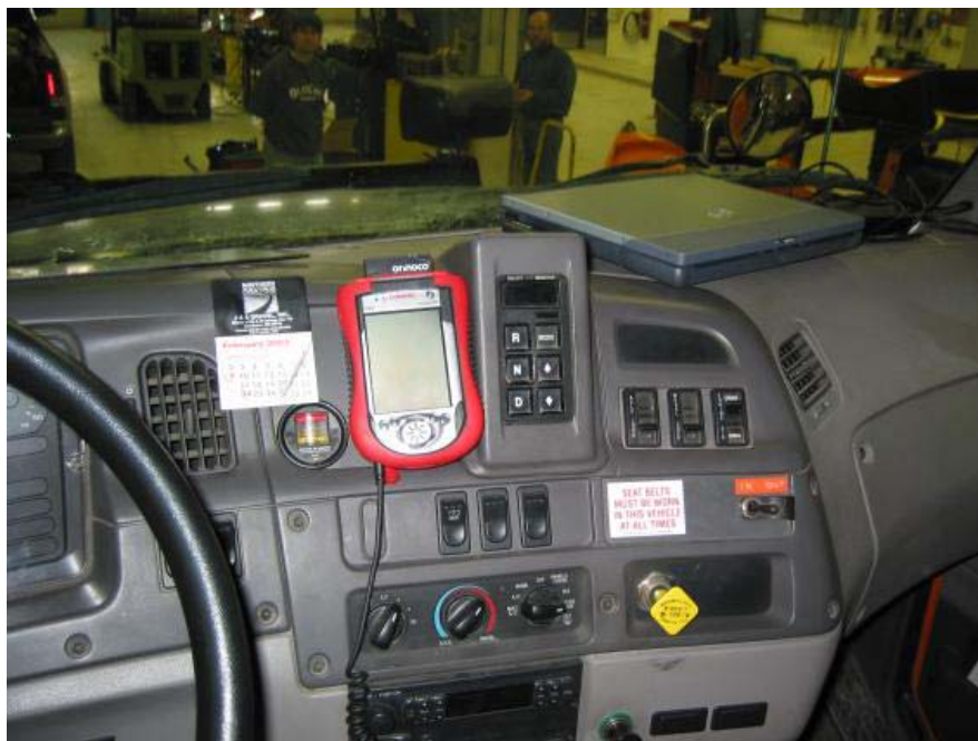
Figure 3.3. View of driver control panel mounted on vehicle dashboard. The control panel is a Compaq iPAQ running IV Lab control panel software.
