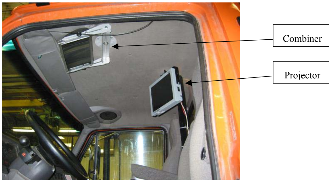
Figure 3.1. Interior view of first Crookston Plow equipped with Driver Assistive system. Combiner is shown in the “up” position.
