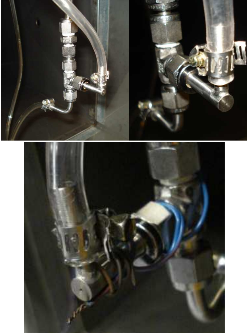
Figure 3.5.1.1: Orifice sampling nozzle installed in sampling section. Thermocouple installed for gas temperature measurement to ensure proper flow calculation.
