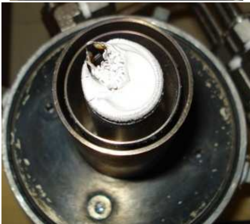
Figure H.14 : SiO 2 cap formed at burner outlet after experimental trial.
