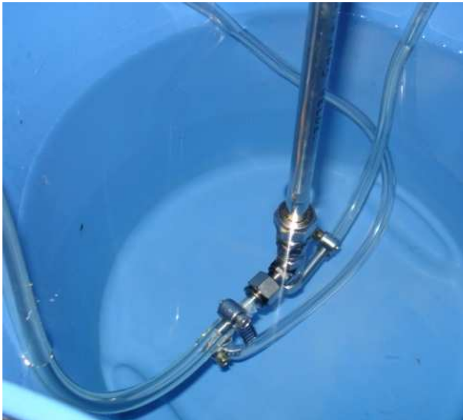
Figure 3.5.1.2: Orifice leak check before, during, and after each calibration experiment.
