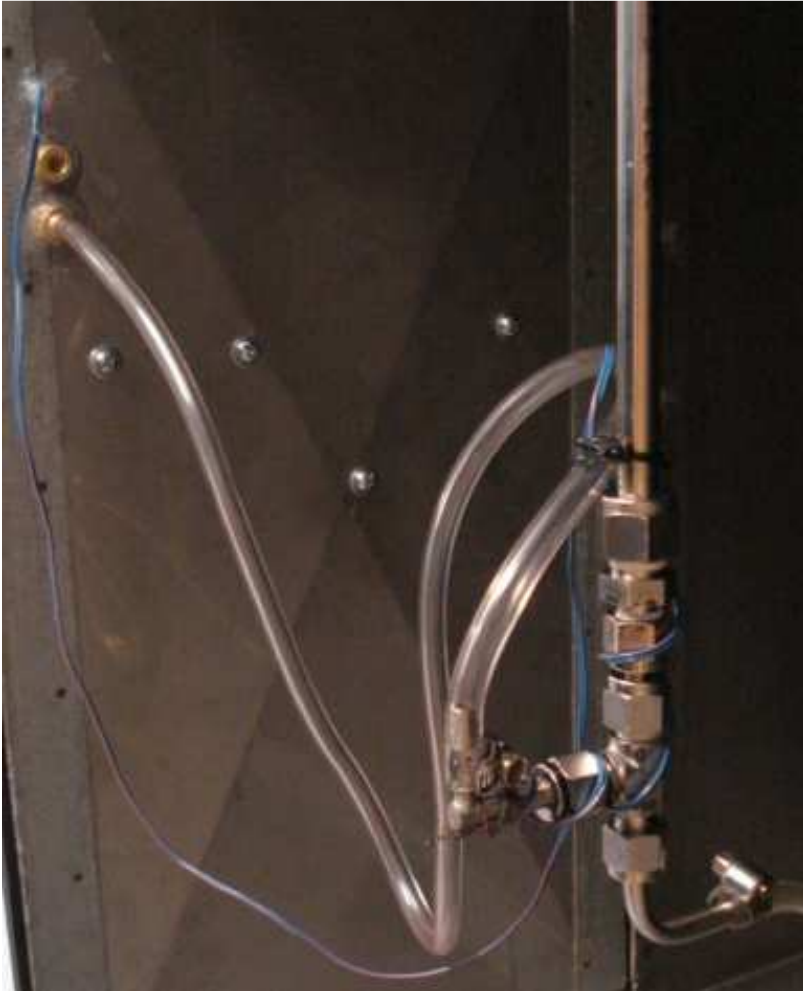
Figure 3.5.1.5 : Final orifice setup with thermocouple.
