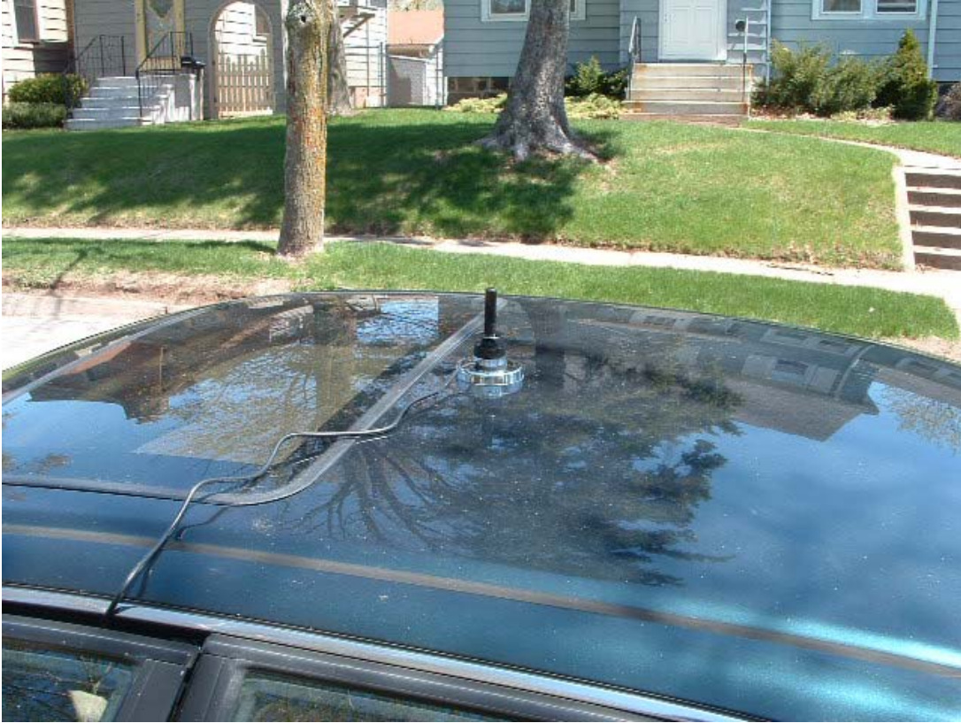
Fig. 2.9 The transmitter antenna magnetically mounted on the roof of a test vehicle.
