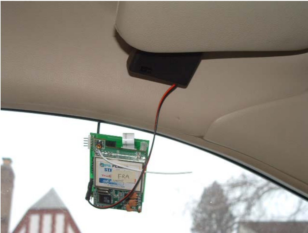
Fig. 2.5 The STXe transmitter module mounted on a test vehicle.
