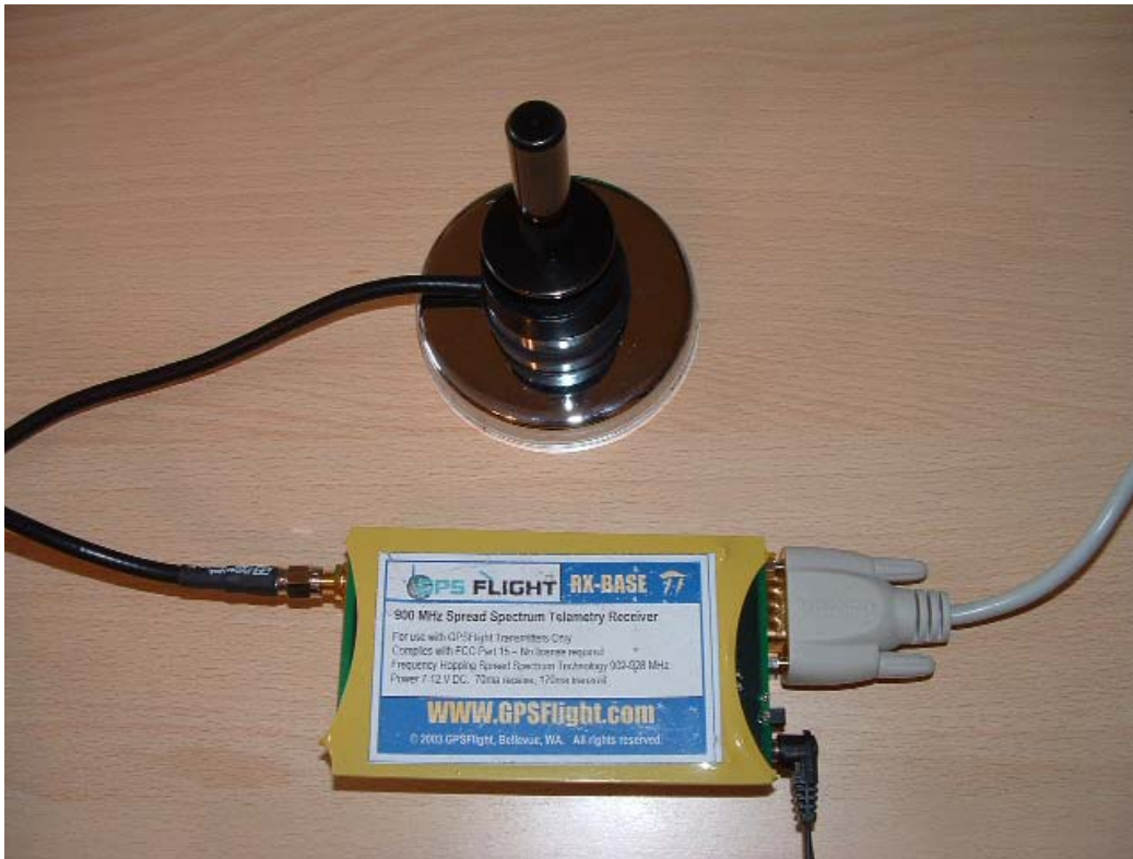
Fig. 2.6 The RX-Base 2 module with a 900 MHz magnetic mount antenna.
