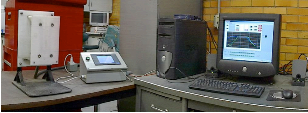
Figure 8: Sensor instrumentation, including FT sample cell and user interface connected to PC running LabView Software.
