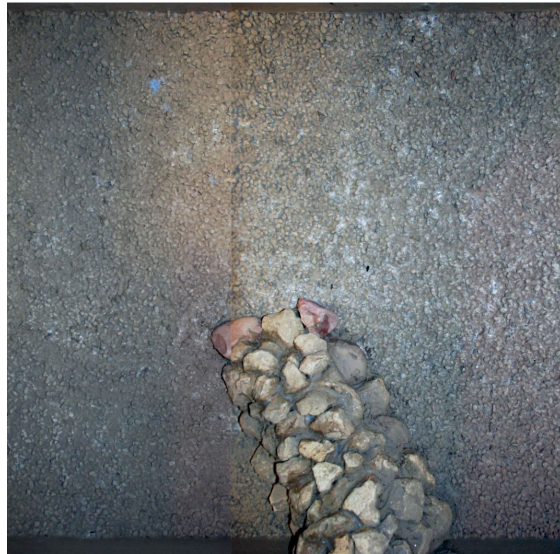
Figure 1.4: Bendway weir installed at the SAFL indoor flume (the flow direction is from left to right; image courtesy of Craig Hill).
