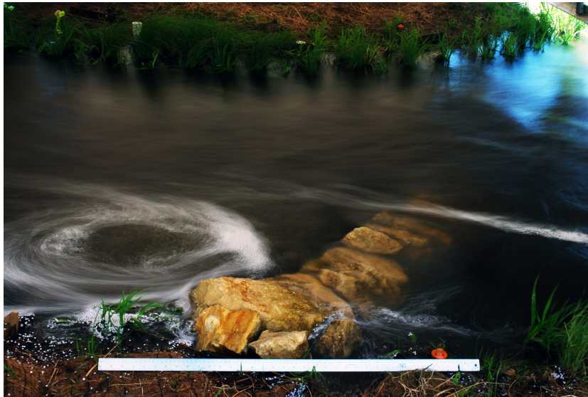
Figure 1.1: A rock vane installed at the SAFL Outdoor StreamLab (the flow direction is from right to left; flow is visualized by tracers, which show formation of a recirculation zone and a shear layer around the rock vane).
