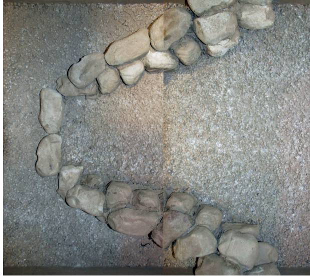
Figure 1.3: A cross vane installed at the SAFL indoor flume (the flow direction is from left to right; image courtesy of Craig Hill).
