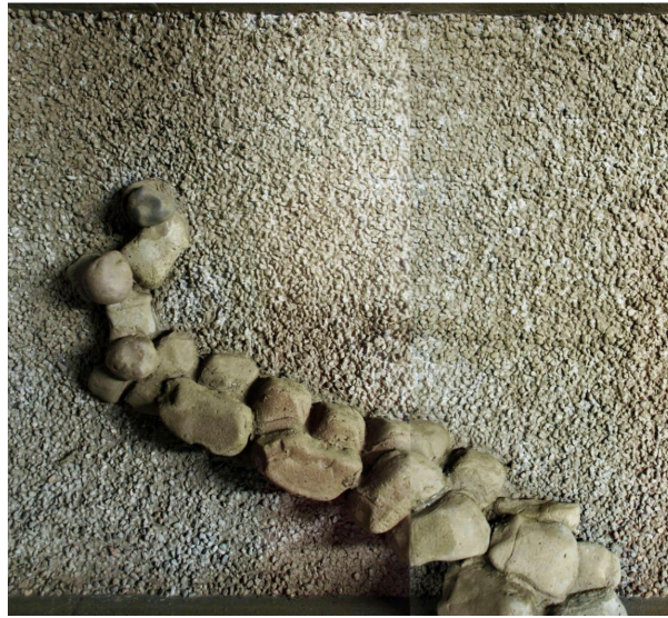
Figure 1.2: A J-hook vane installed at the SAFL indoor flume (the flow direction is from left to right; image courtesy of Craig Hill).
