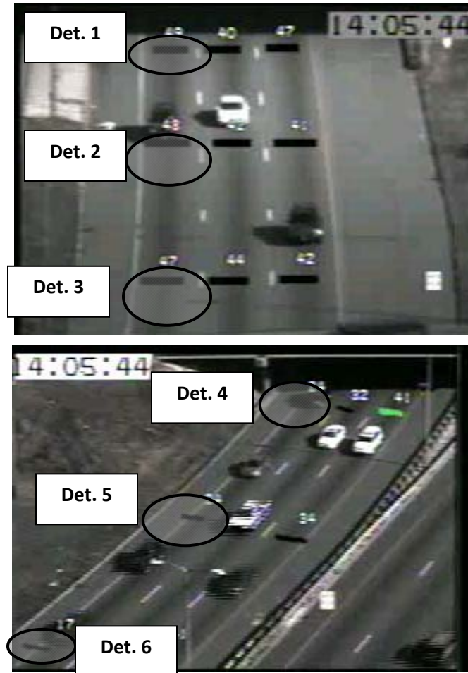
Figure 3. 10 Successive detector Locations used at two zones to estimate speed profile
