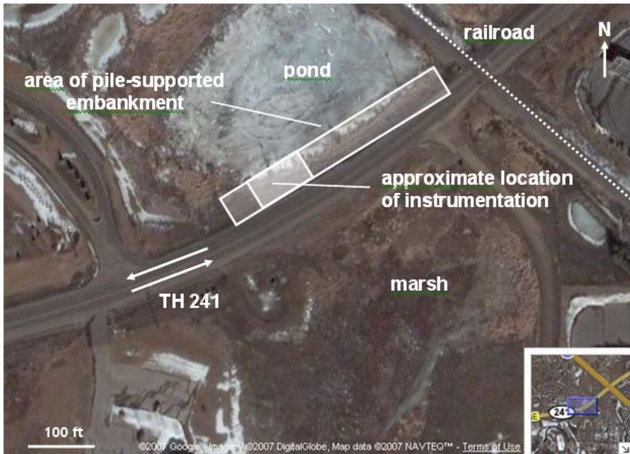
Figure 3.2. Plan view of site prior to highway expansion. Note the close proximity of the BNSF railroad to the pile-supported area.
