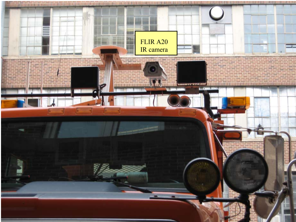
Figure 4. FLIR A20 IR camera on the Safeplov
