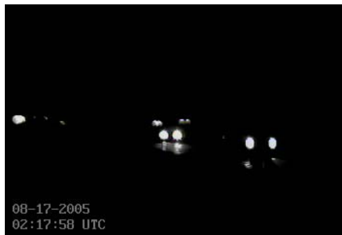
Figure 2. A captured image from a Panasonic WV-CL920V camera. It is difficult to determine if two light blobs belong to one or two vehicles or motorcycles.
