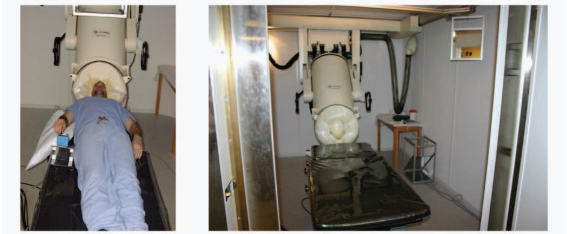
Figure 5.2: Left: The 248-sensor whole-head MEG system is located inside a shielded room that reduces electromagnetic and environmental noise. Right: The subjects lay supine in the recording chamber with their heads inside the cryogenic helmet-shaped dewar. The joystick was mounted comfortably at arm's length on the right side.
