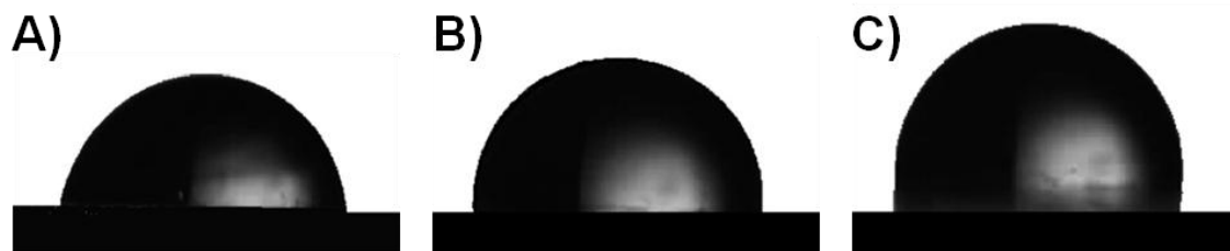
Figure 2.21. Water droplets from contact angle measurements for A) neat epoxy, B) 20 wt % and C) 40 wt % PTFEA-PEO block polymers. (adapted from Yi et al.) 65
