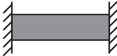
Figure 6.1: Geometry for a problem of a restrained bar.
