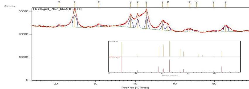
Above: X-ray diffraction plot for the solution synthesized in milli-Q water after aging. The rest of the solutions closely match the same profile after aging, with the exception of the solution aged in 0.1mM Alizarin.
