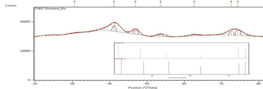
Above: X-ray diffraction plot for the solution synthesized in milli-Q water before aging. The rest of the solutions closely match the same profile before aging. The solution aged in 0.1mM Alizarin also matched this profile.
