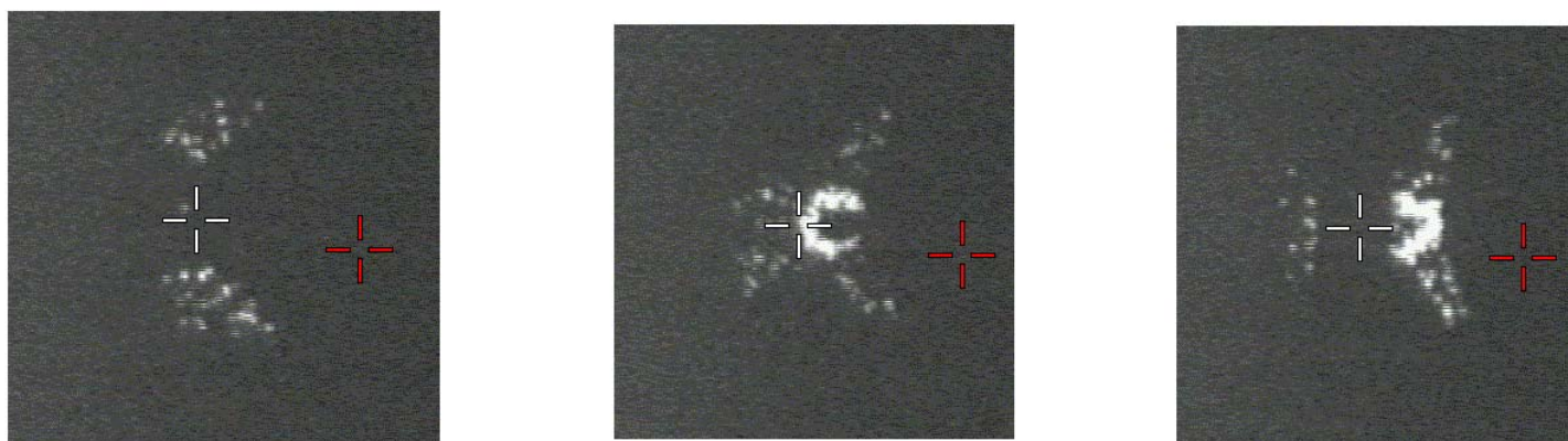
Figure 2.3. ^{19}\text{F}^- secondary ion image on indium, which illustrates the secondary ion optic axis (located with the white reticle). The center image has the mass adjusted by the secondary magnets to maximize the count rate. The left image is that of when the secondary magnets are adjusted to a decreased mass (vertically pinching out), while the right image is that of when the secondary magnets are adjusted to an increased mass (horizontally pinching out). It can be seen in the center image that the primary ion beam is generating secondary ions slightly to the right of the secondary ion axis. Steering of the primary magnets can re-align the primary ion beam to produce secondary ions with the greatest count rate when the secondary magnets are aligned directly over the secondary ion axis.
