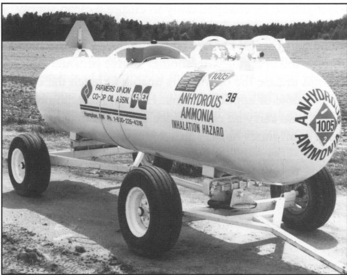
Paint anhydrous ammonia tanks white to prevent rusting and to help keep the temperature and pressure down inside the tank during warm weather.
