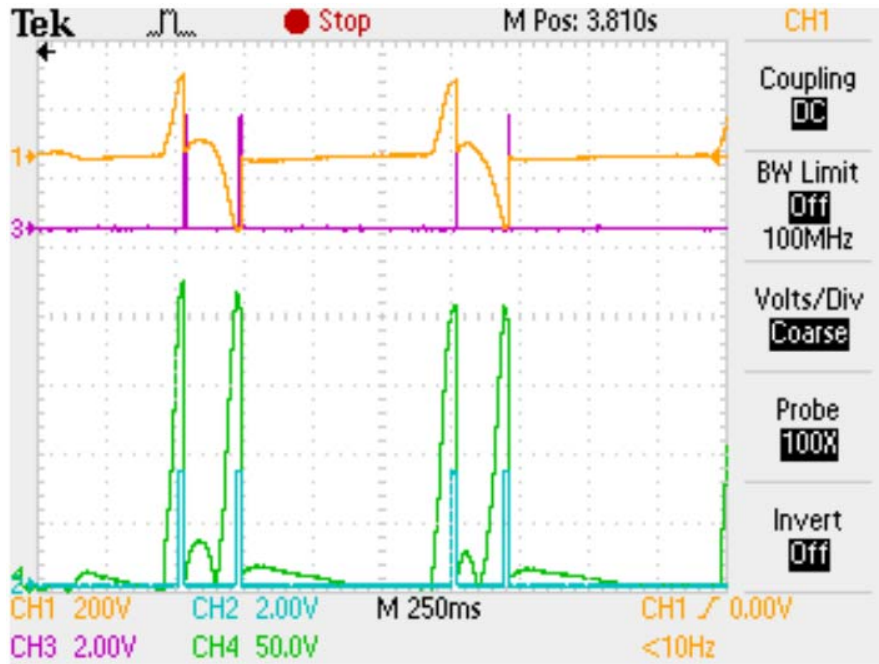
Figure 7.4: Rectified (CH4) and unrectified (CH1) source output signals, note CH1 is 200V/division, with comparator output (CH2) and switch close signal (CH3)
