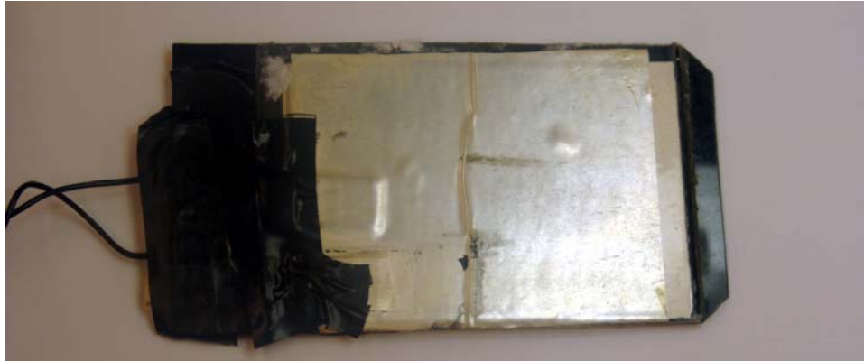
Figure 4.7: 8-layer PVDF Nylon Insole with 3M Double Sided Tape as Adhesive
