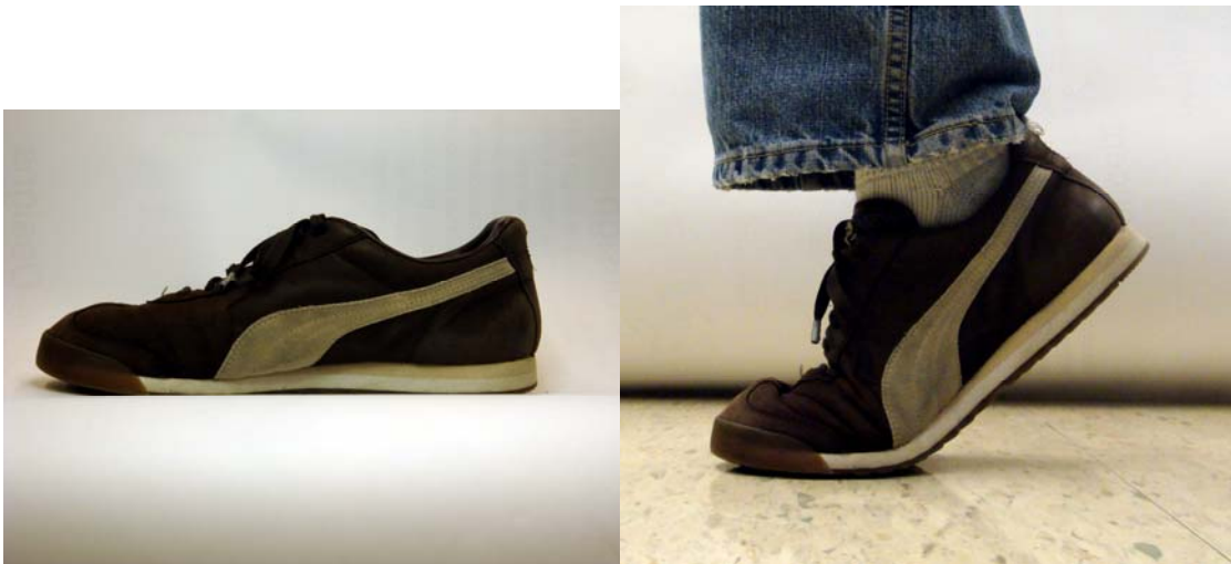
Figure 3.3: Street Shoe with Flat Toe and Bending During Propulsive Phase
