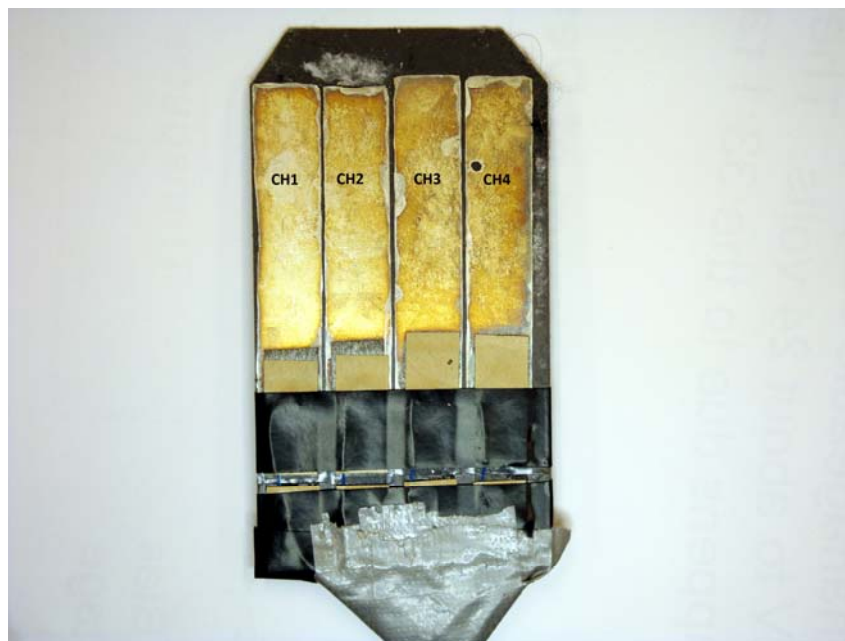
Figure 3.6: PVDF Insole Strip Test for Optimum Width
