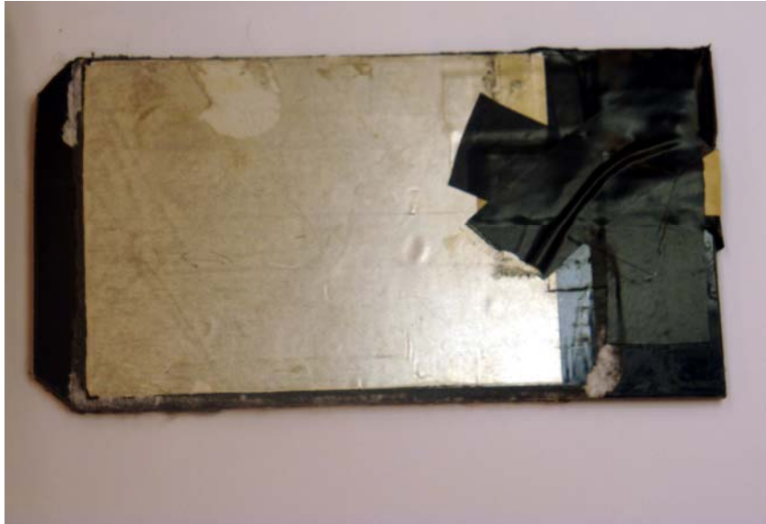
Figure 4.9: 8-layer PVDF Nylon Insole with 3M DP-105
