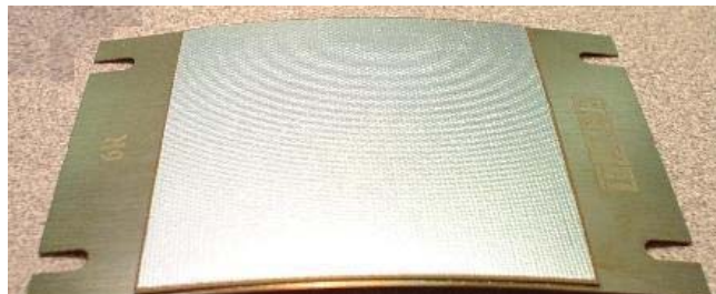
Figure 2.3: Thunder Construction (Top) and actual Thunder TH-6R unit.
