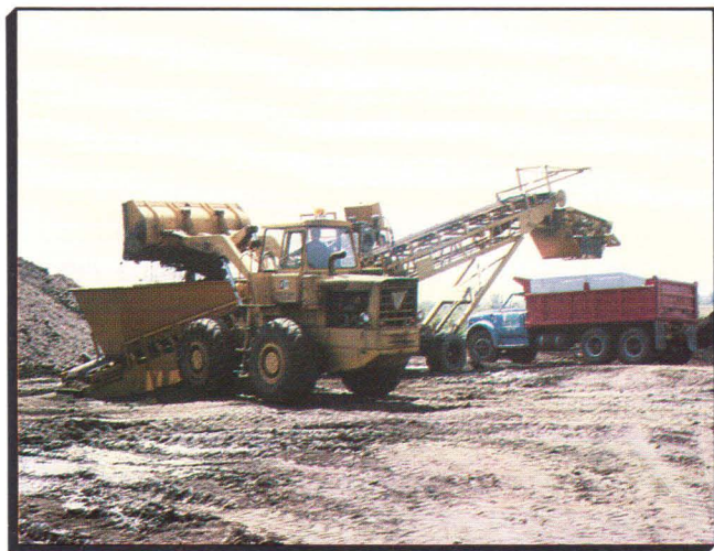
Figure 6. A mixer-shredder to prepare soil mixtures for athletic fields.
