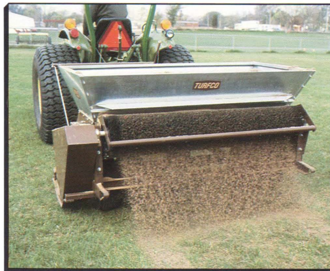
Figure 12. Topdresser for surface application of thin soil layer.
