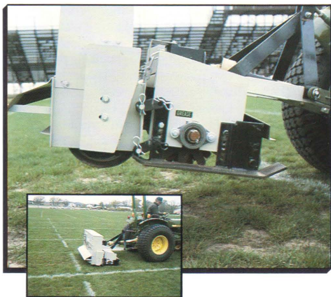
Figure 11. Slit seeder for initial establishment and overseeding.
