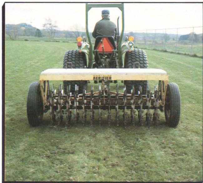
Figure 10. A core aerifier for athletic turf removes soil cores to relieve compaction and reduce thatch build-up.
