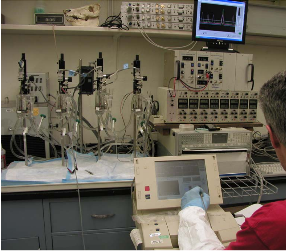
Figure 4. The experimental test apparatus showing 4 of the 8 tissue baths, the temperature control system (back, left side), eight force transducer outputs and computer monitor, and the Medtronic Pacing System Analyzer.
