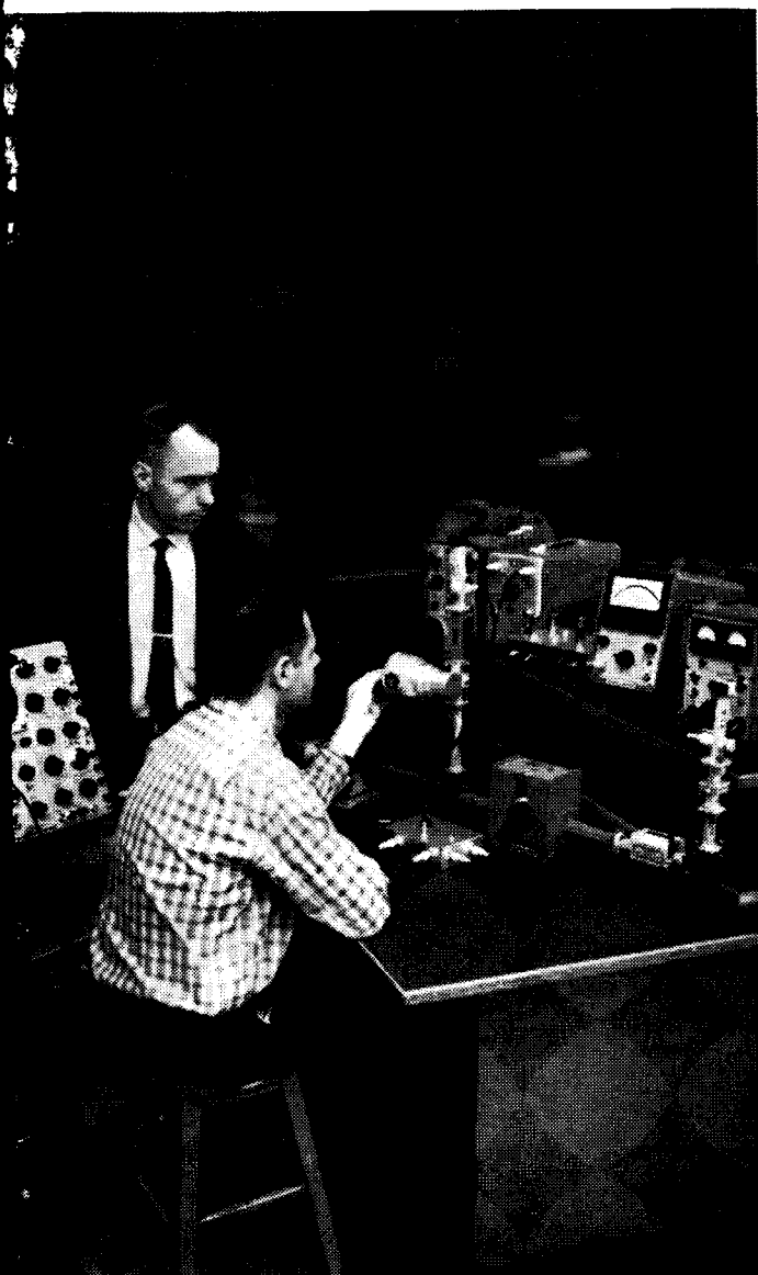
Student measuring the electrical properties of a semiconductor crystal with microwaves.
