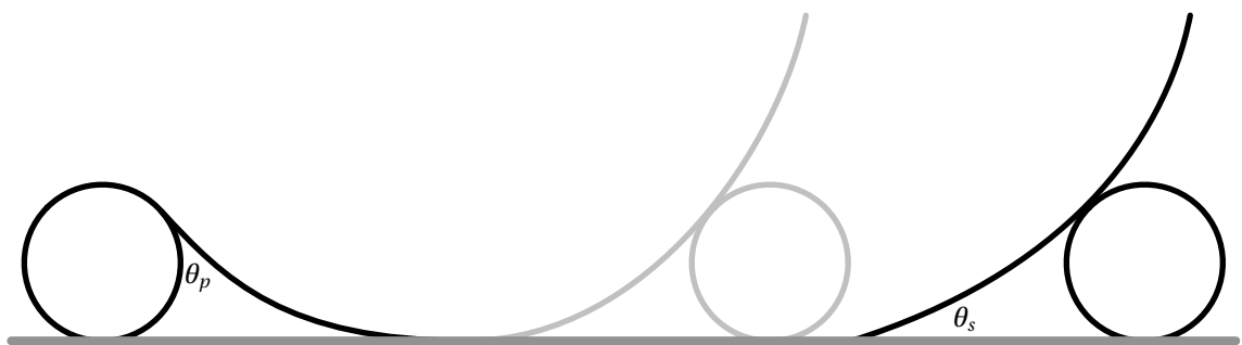
Figure 4.11: Static model for inter-band spacing with consideration for liquid-substrate contact angle. A finite contact angle \theta_s after a meniscus “breakage” implies an equilibrium capillary rise smaller than for zero-contact angle, and the predicted inter-band spacing \lambda will consequently be larger.
