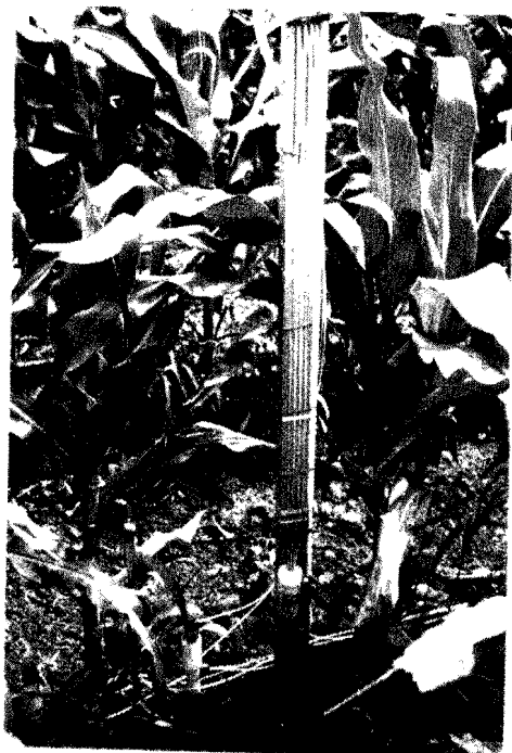
Tensiometer manometers give soil water potentials in soils to 2 meter depths.
