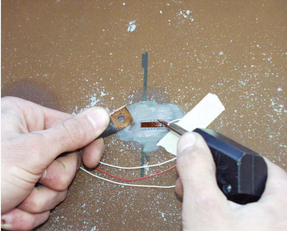
**Figure 3.1: Welding of a strain gage**
