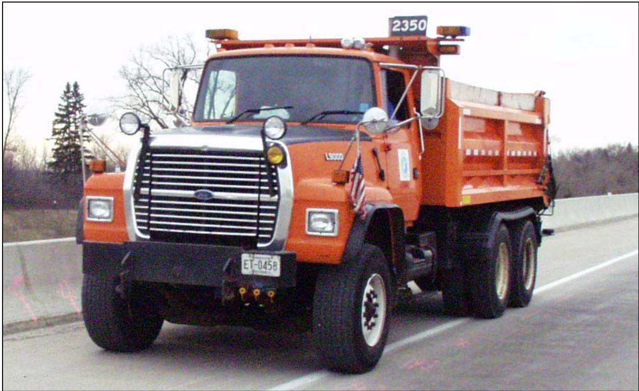
Figure 3.7 Typical 3-axle Mn/DOT truck used for live load tests
