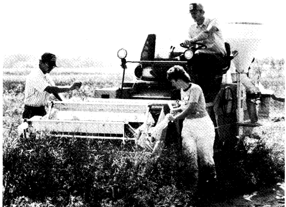
Agronomist Dan Putnam maneuvers a small-plot combine harvesting spring planted canola. Student technicians on the ground assure that the plant material feeds smoothly and is completely harvested.
