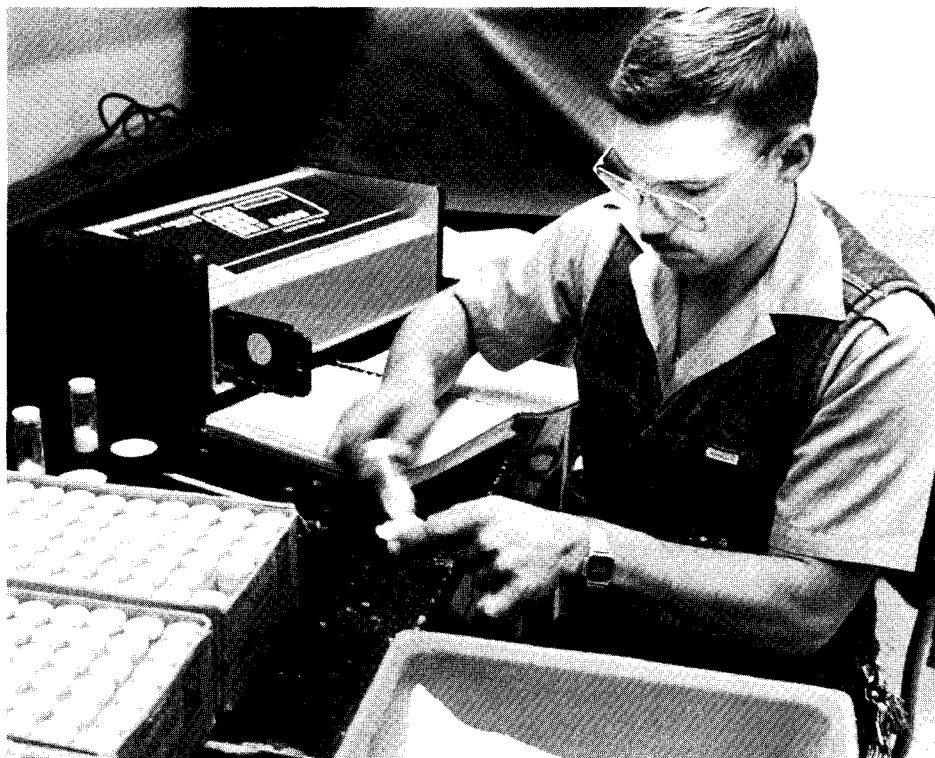
Soybean meal samples are run through a near infra-red analyzer to determine oil and protein content. Technician Neal Batt fills sample cells from 65-gram portions of ground soybean seed.
