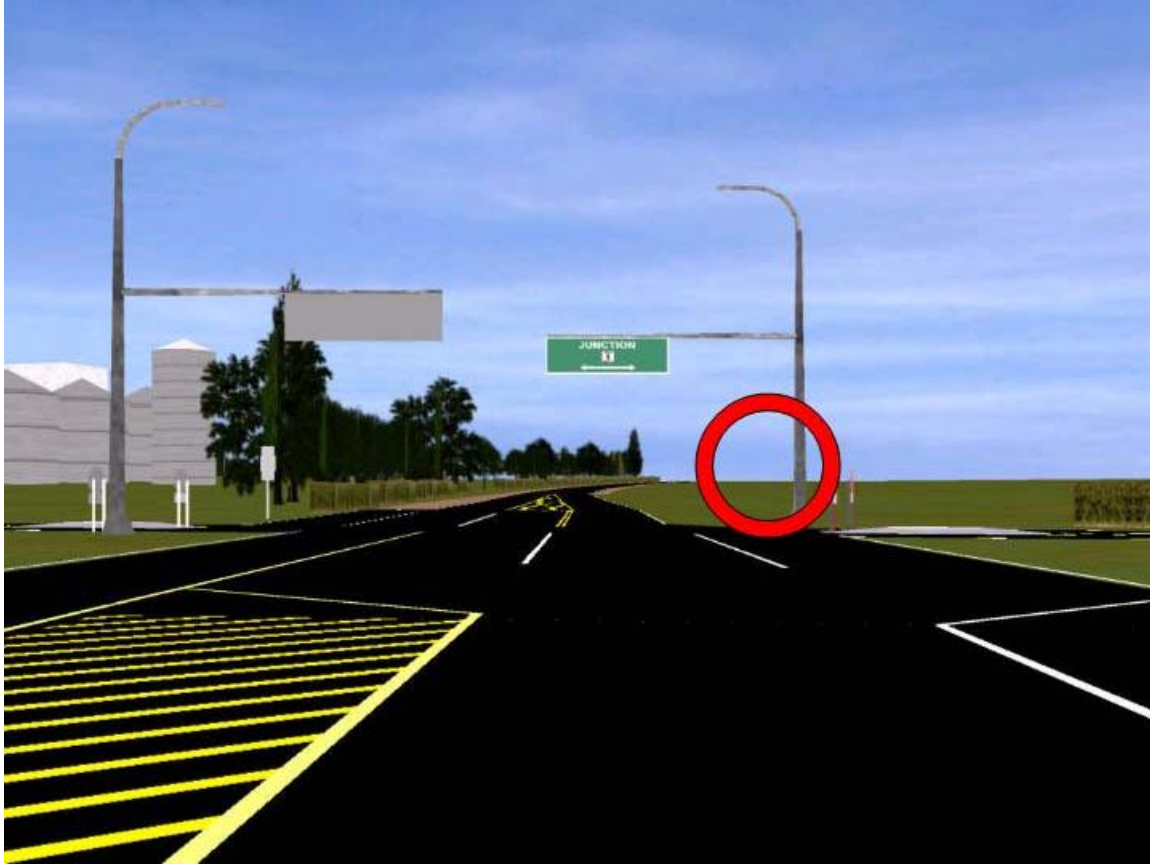
Figure 2.7. Simulated After Condition, with the Vegetation on the Eastside of the Approach from the North (Viewed from the South) Removed from the Area Circled in Red
