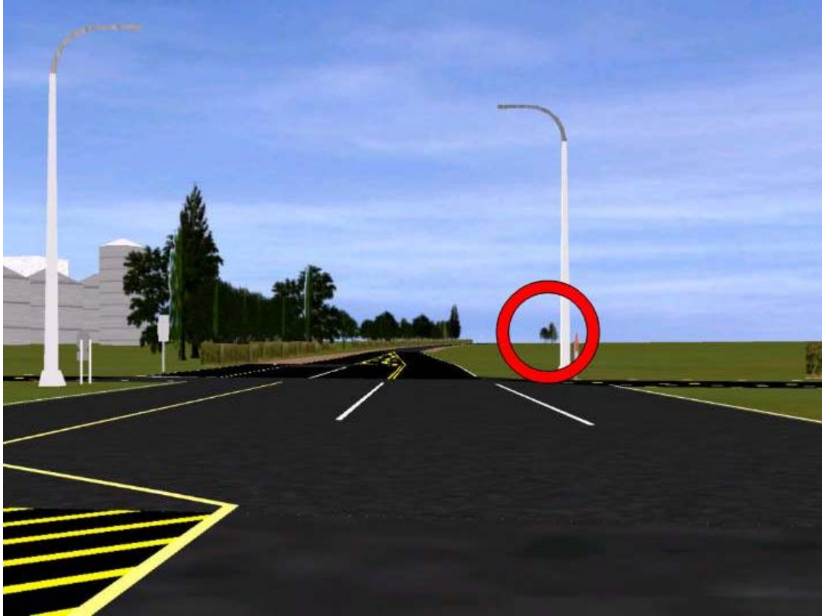
Figure 2.6. Simulated Before Condition, with the Vegetation on the Eastside of the Approach from the North (Viewed from the South) Circled in Red
