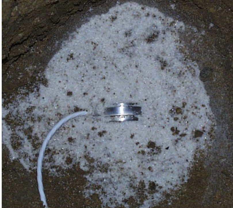
Figure 3.6. Kulite EPC within sand pocket.
