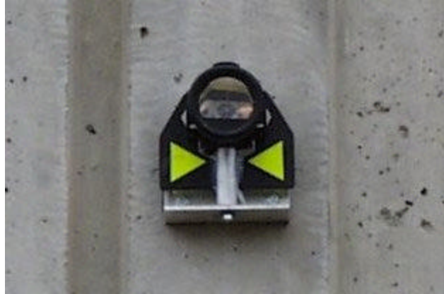
Figure 3.11. Prismatic survey reflector fastened to front face of the wall.
