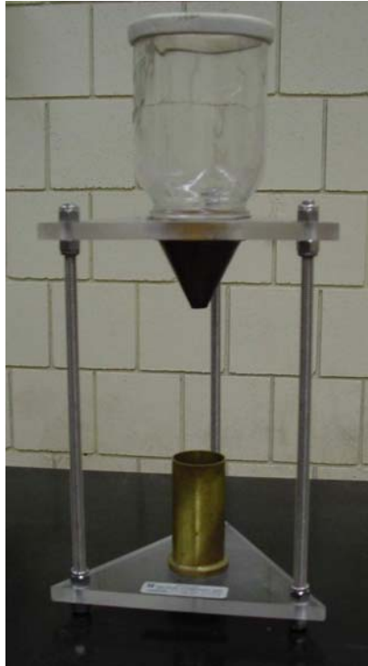
Figure 4.1 Standard testing apparatus for AASHTO T304, ASTM C1252 Method A
