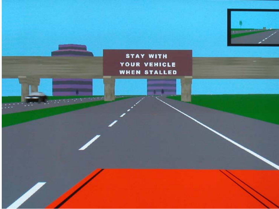
Figure 2.4. Overpass with Category III CMS Message.
