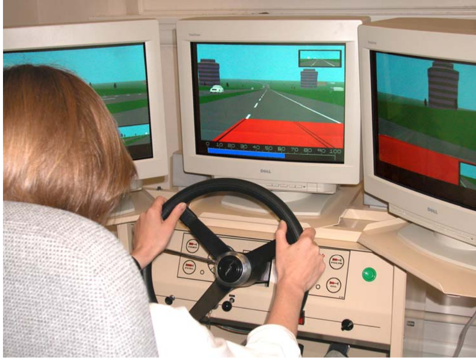
Figure 2.1. The STISIM Driving Simulator used in this experiment.
