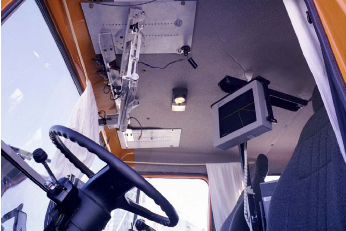
Figure 4. Interior view of snowplow—taken from doorway. The figure shows the Head-Up Display above the steering wheel, and the projection display up and to the left of the driver's seat.
