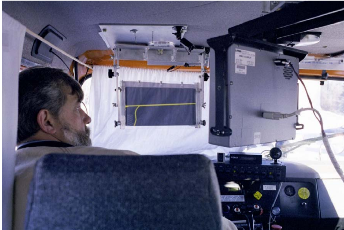
Figure 3. Interior view of snowplow—taken over the shoulder of an operator. The figure shows the Head-Up Display directly in front of the curtains used to occlude the view through the windshield. The projection display used to provide the image seen on the Head-Up Display is in the upper right foreground of the picture
