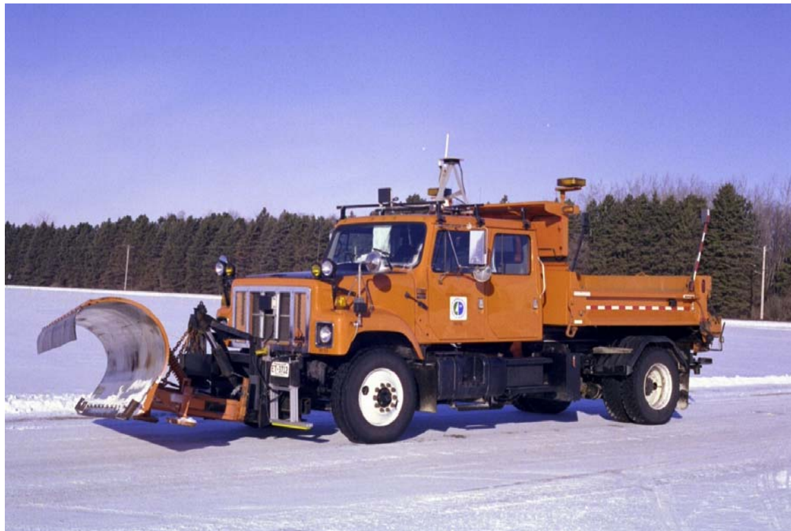
Figure 1. Snowplow equipped with Driver Assist System at Rosemount Test Site. The aerial used for satellite transmissions can be seen on top of the vehicle's cab
