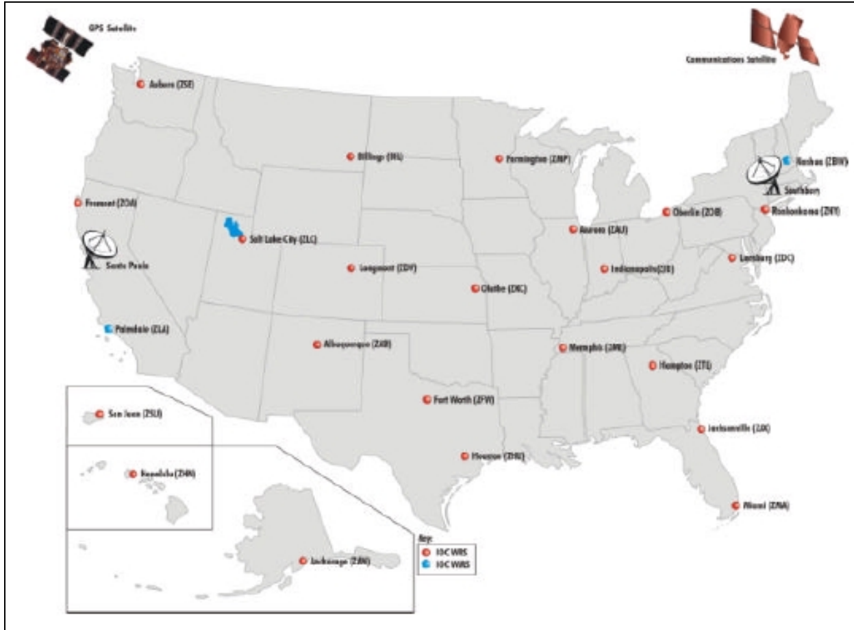
Figure 3.4 WAAS architecture and the network.
