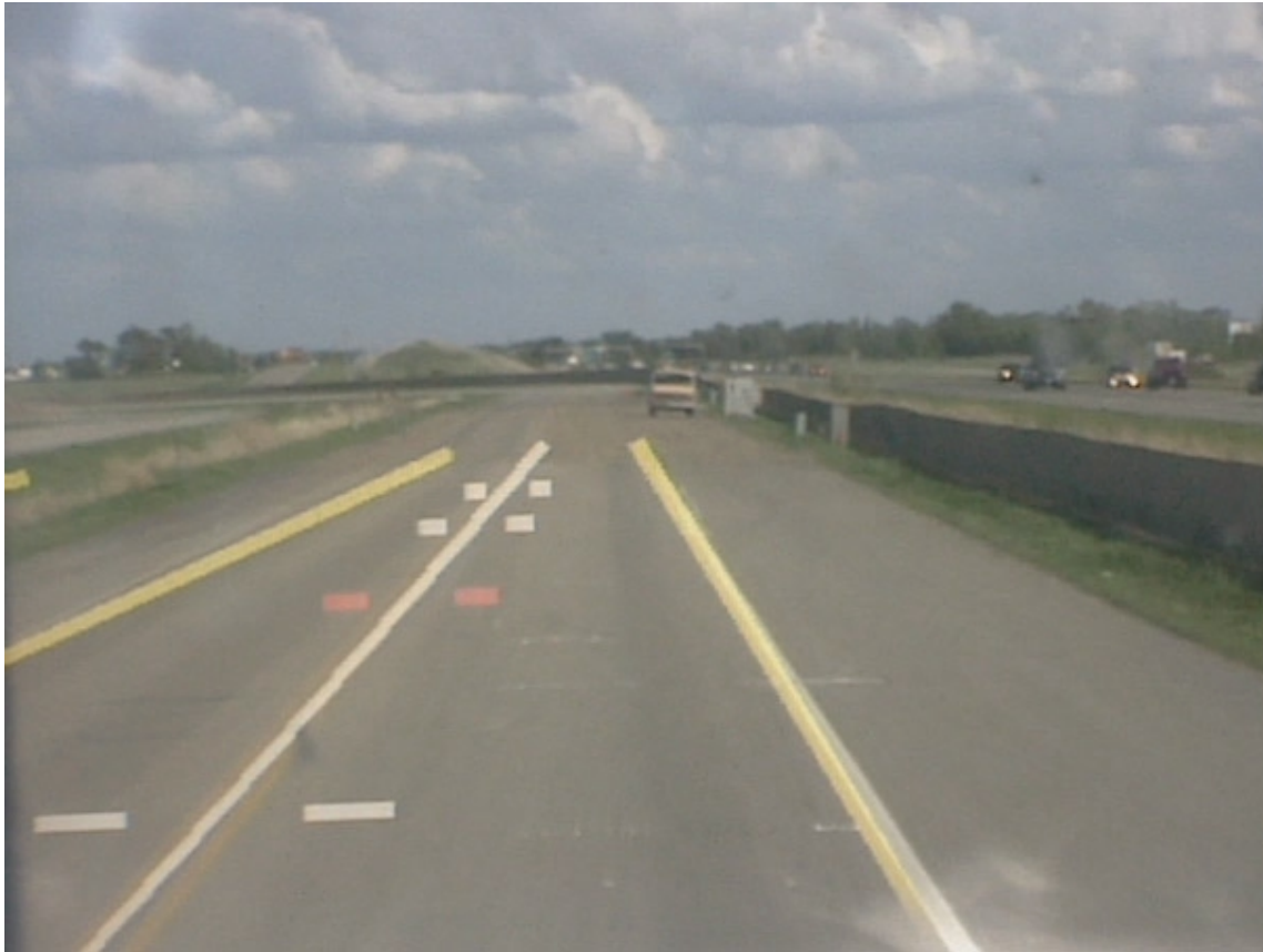
Figure 5.2 Yellow lane boundaries and white center line from the database are superimposed over actual lane markings as a demonstration of accuracy. The short horizontal bars are superimposed for calibration and evaluation purposes and are not typically used.
