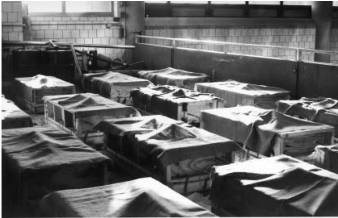
Figure 2.9 Concrete Specimen Forms with Burlap
