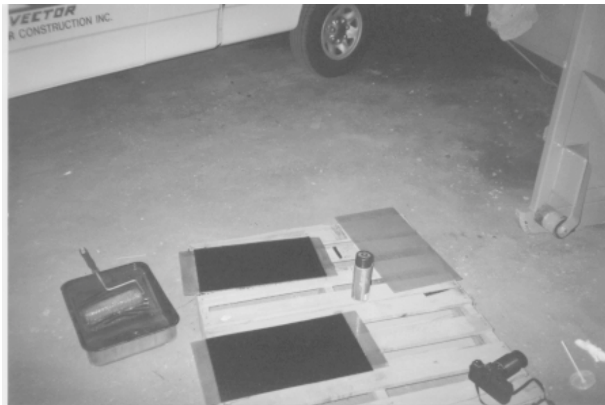
Figure 3.21: Fabrication of diffusion test specimens of MBrace CFRP composite
