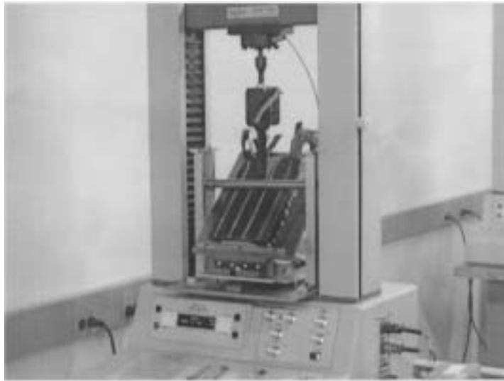
Figure 6.10: Peel test of MBrace composite in progress on SATEC load frame
