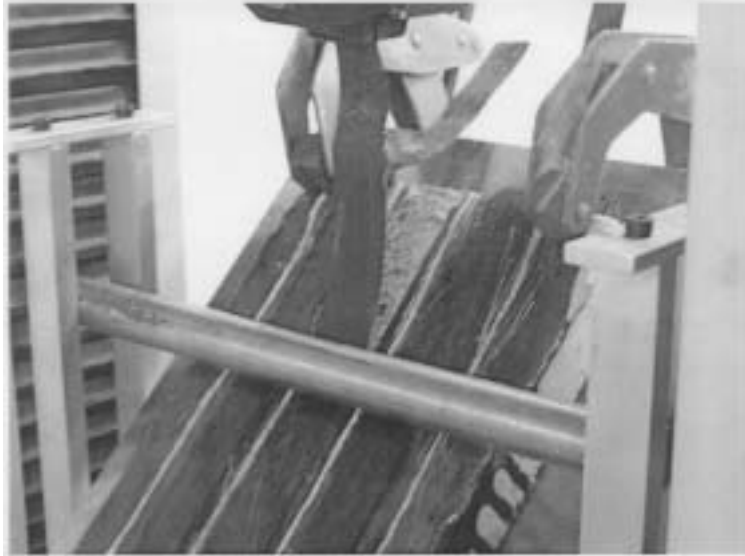
Figure 6.13: Peel test of MBrace CFRP wrap
