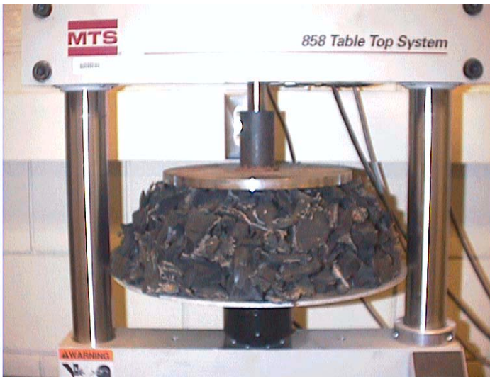
Fig. 3.2. MTS load frame setup a) constrained compression b) unconstrained compression
