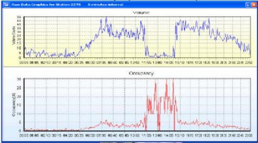
Figure A.15 An unusual data error that can not be properly filtered
