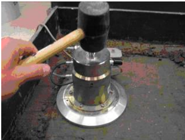
Figure 2.15: Rubber mallet tapping the modified LWD
