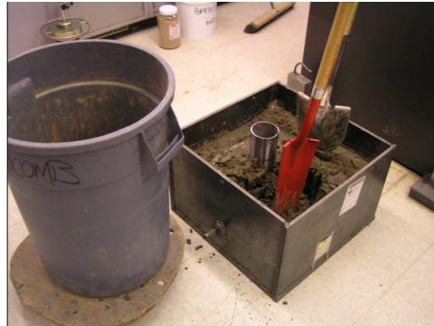
Figure 4.17: a) Stainless tubes and b) specimen extraction
