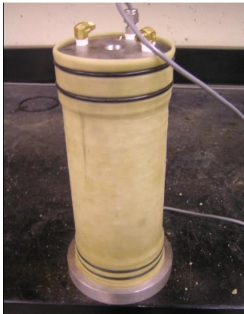
Figure 2.5: Specimen placed inside rubber membranes
