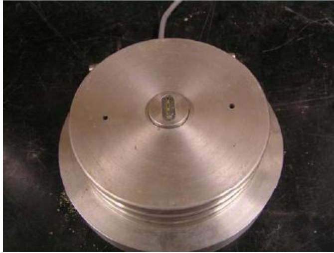
Figure 4.19: Lower platen housing bender element
