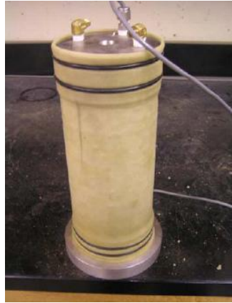
Figure 4.20: a) Encased soil specimen and b) LVDTs collar-type holder
