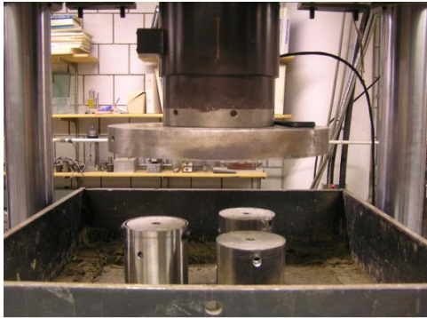
Figure 4.17: a) Stainless tubes and b) specimen extraction
