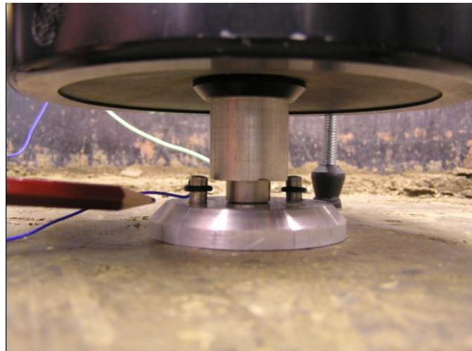
Figure 2.20: PVD loading plate in contact with soil
