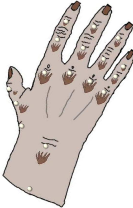
Figure 2.5. Placement of reflective markers. Markers were placed close to, but not directly on each joint.
