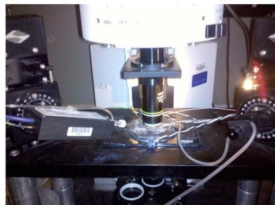
Experimental setup. The slice is placed in the center underneath the microscope, with the electrode mounted in the holder on the left. The image is projected onto a television screen (not shown) for better view.
