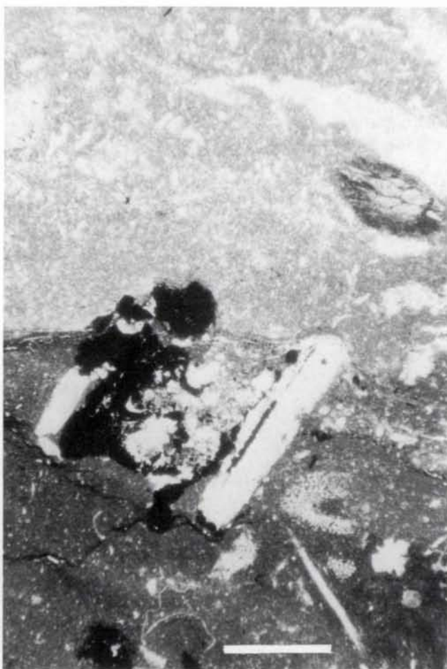
Figure 14. Idiotopic dolomite crystals. Note euhedral to subhedral crystal shapes and straight intercrystalline boundaries. Bar scale is 0.5 mm long.
