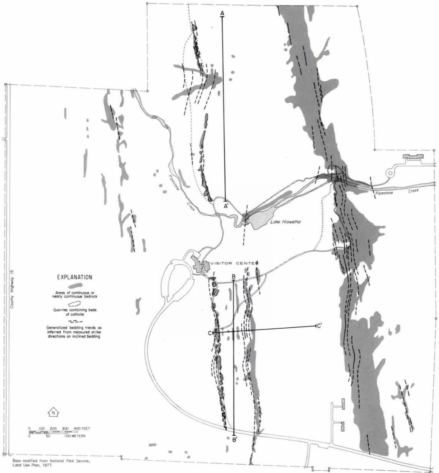
Figure 5. Trend lines of master bedding planes in the Sioux Quartzite as inferred from the structural data of Figure 4. Note also the curvilinear rather than planar nature of these structures. See Figure 6 for cross sections A-A' and B-B' and Figure 7 for cross section C-C'.
