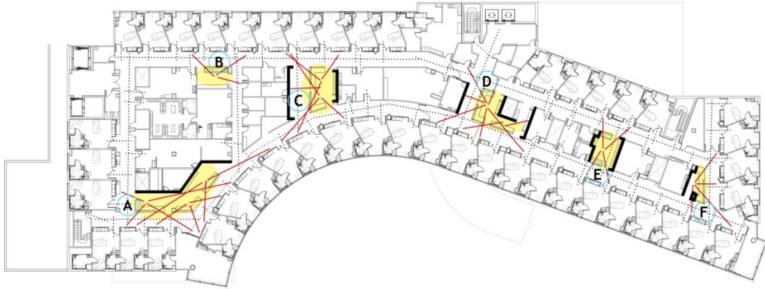
Figure 19. Plan A: Centralized medical-surgical nursing unit model with six pods, each with a varying number of patient rooms. Nurse stations vary in size and in proximity to patient rooms and to each other.
