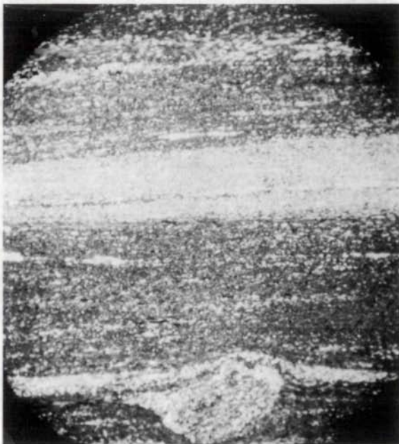
Figure 13 - Photomicrograph of thin compositionally-different laminae in intermediate tuff from drill hole BD-1. Amphibole-rich (broad medium-gray bands), biotite-rich (thin dark gray bands) and feldspar-quartz-rich alternations; one garnet crystal at left. Field of view is 5 mm across.
