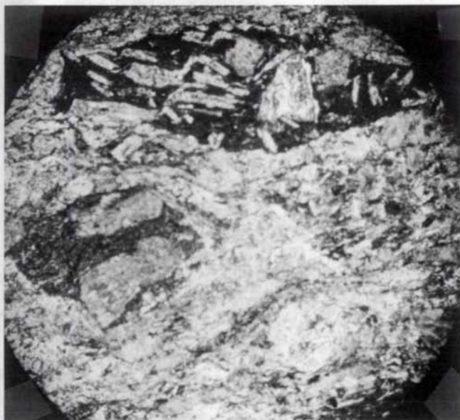
Figure 9b - Photomicrograph of volcaniclastic rock from N 1/2, Section 10, T.159N., R.28W. Note varying textures and colors of volcanic rock fragments. Field of view 5 mm in diameter.
