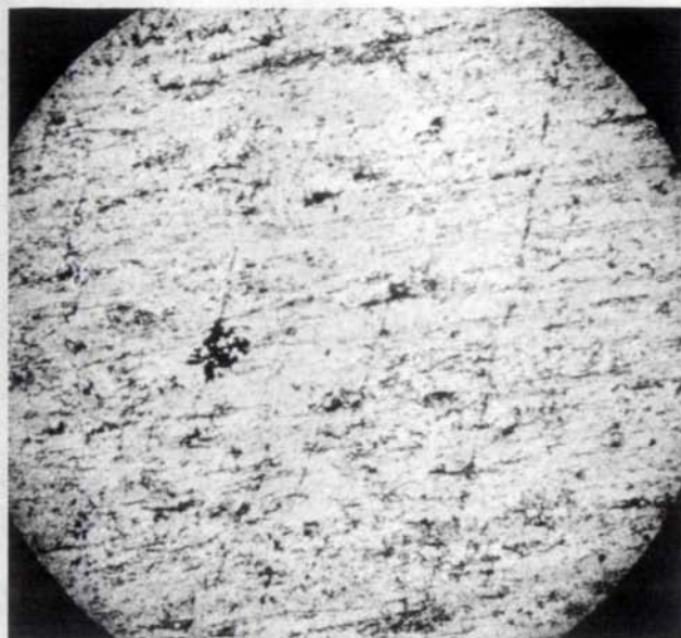
Figure 16 - Photomicrograph of felsic tuff with two foliations, from NW 1/4 Section 6, T.159N., R.25W. Field of view 5 mm across.
