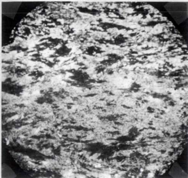
Figure 8a - Photomicrograph of possible shards from felsic-intermediate tuff exposed along Manitou Rapids dike in Section 6, T.159N., R.25W. Field of view 5 mm in diameter.
