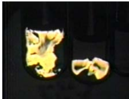
Fig.5.3. Intermediate birefringent liquid crystals at T = 45 [°C] for the CsDS/water system; left , 38 wt % CsDS; right , 20 wt % CsDS. Heating rate larger than 0.2 [°C/min], starting from T = 25 [°C]. Cross-polarized light was used. Size scale : tube diameter is 15 [mm].
