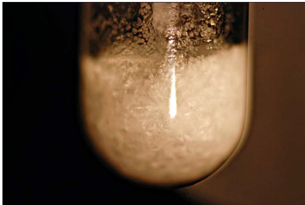
Fig.4.7. Initially supercooled sample. Initially heated from T = 25 [°C] to T = 55 [°C] with a heating rate higher or equal than 0.2 [°C/min]. Then, the sample was cooled down to 0 [°C] for an hour and then brought again at T = 25 [°C] to warm naturally). Figure captured at T = 25 [°C] after natural warm - up. No cross-polarized light was used. Size scale , tube diameter: 15 [mm].
