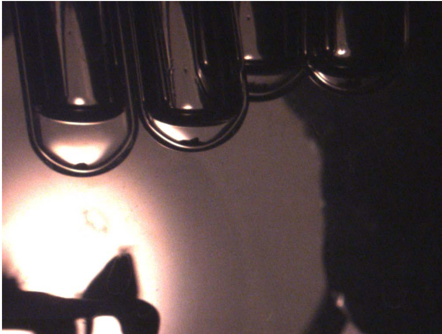
Fig.C.2. 5%, 10%, 15%, 20 wt % impure CsDS at T = 31.7 [°C] ( 12^\circ ) - 2 nd heating cycle. Heating started at T = 25 [°C] with heating rate 0.2 [°C/min]. No cross-polarization. Size scale: the tube diameter is 15[mm].
