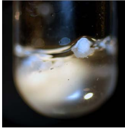
Fig.4.8. Initially superheated sample (from T = 25 [°C] to T = 55 [°C] with a heating rate higher or equal than 0.2 [°C/min] and then naturally cooled to T = 25 [°C]). Figure captured at T = 25 [°C] after natural cool down. Size scale , tube diameter: 15 [mm]. No cross-polarized light was used. Solid crystals form at the boundary of the seed.
