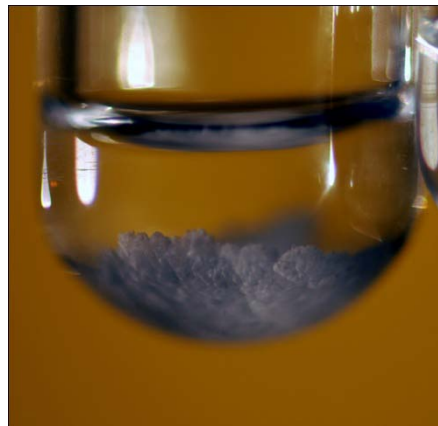
Fig.C.7. Solid crystals (stable state) that have been created at T = 25 [°C] by solute or solvent jump in a 10 wt % CsDS solution (see solvent jump in [87], [35], [36], [37], [90]). Figure captured at T = 25 [°C]. No cross-polarized light was used. Size scale: the tube diameter is 15[mm].
