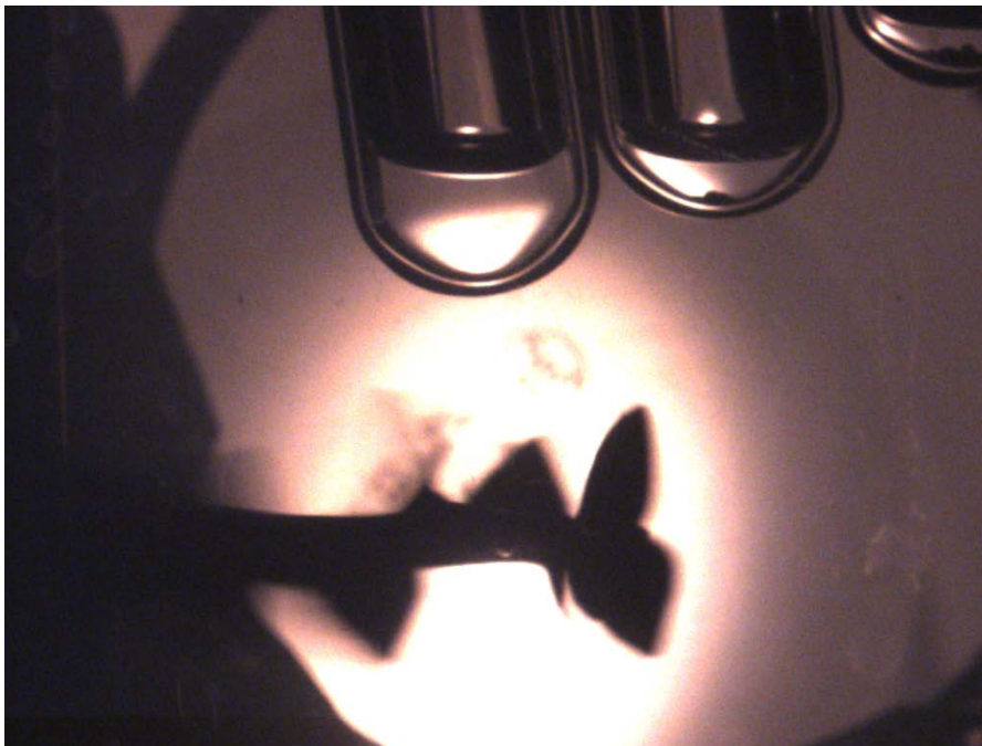
Fig.C.3. 5 wt % and 10 wt % impure CsDS at T = 32.1 [°C] - seed is melting. Heating started at T = 25 [°C] with heating rate 0.2 [°C/min]. No cross-polarization. Size scale: the tube diameter is 15[mm].
