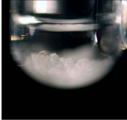
Fig.C.8. Solid crystals (stable state) created by solute or solvent jump in a 20 wt % purified CsDS solution after heating, at T = 25 [°C] (see solvent jump in [87], [35], [36], [37], [90]). Figure captured at T = 25 [°C]. No cross-polarized light was used. Size scale: the tube diameter is 15[mm].
