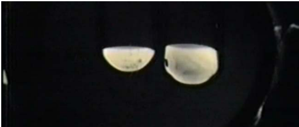
Fig.5.6. 30 wt %, 15 wt % purified CsDS at T = 48 [°C]. Intermediate, birefringent liquid crystals are observed in both samples. Heating rate higher than 0.2 [°C/min], starting from T = 25 [°C]. Cross-polarized light was used. Size scale : tube diameter is 15 [mm].
