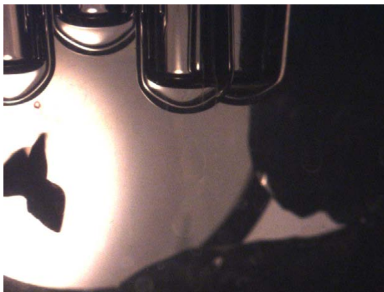
Fig.C.4. 5%, 10%, 15%, 20 wt % impure CsDS at T = 32.4 [°C], (2 nd from right) is a 15% CsDS micellar solution. Heating started at T = 25 [°C] with heating rate 0.2 [°C/min]. No cross-polarization. Size scale: the tube diameter is 15[mm].
