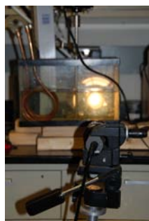
Fig.2.3. Instrument setup of the macroscopic observations. Size scale: The height of the water tank is 8 [inches] and the width is 12 [inches].
